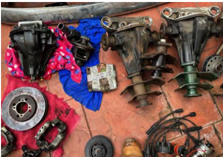
Diffs 3.7, 4.1. 4.1 has chipped tool on crown wheel
