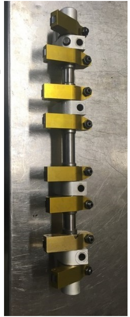
Roller rockers mounted on tuft-ridged shaft with custom bronze bushes (modified for critical oil flow) and solid spacers.
