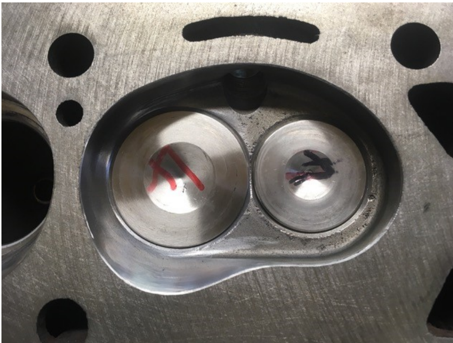
Reshaped chambers to remove shrouding of inlet valves and exhaust valve inserts blended into valve throats..
