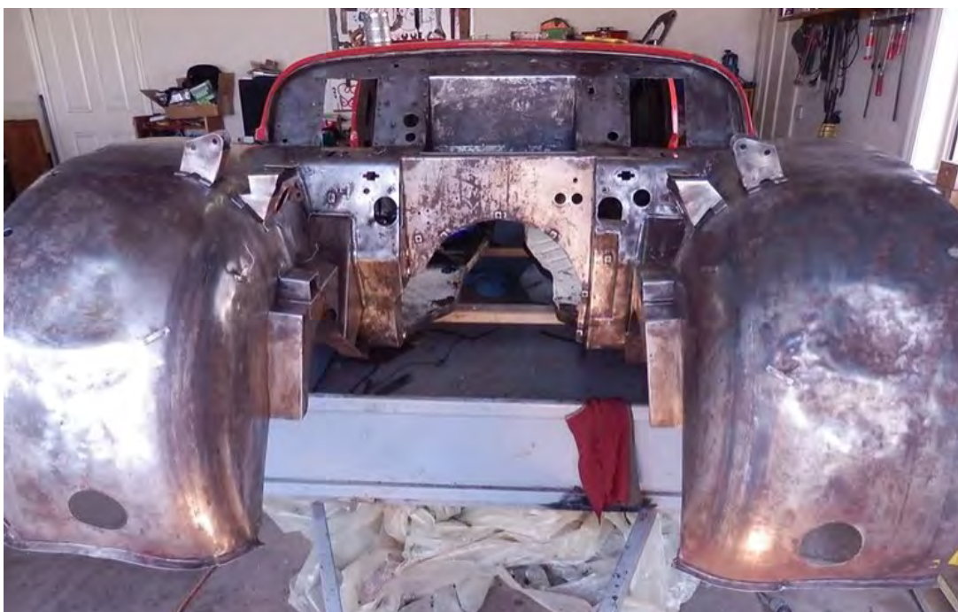
Cleaning the sound deadener spray off the engine bay and everywhere else. Amazing what you can hide under that stuff.
