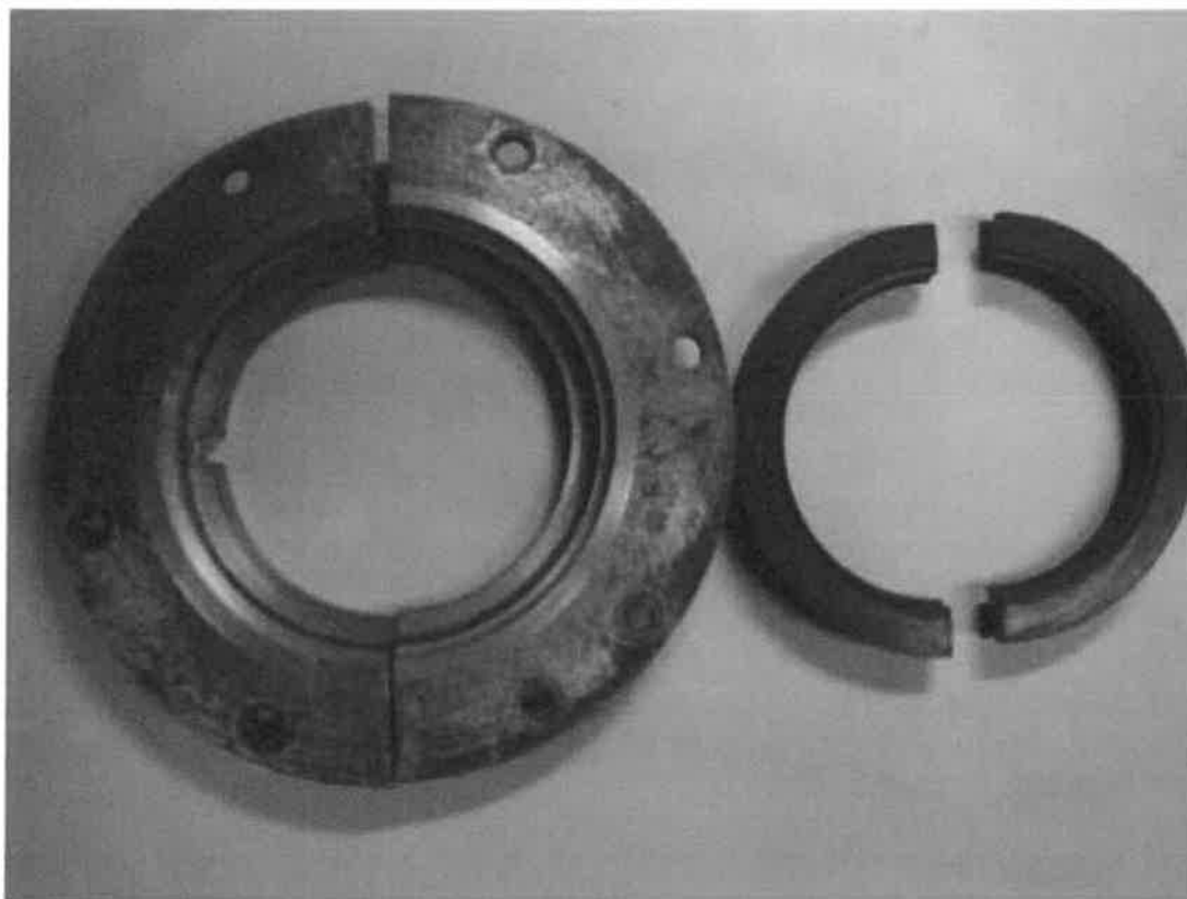
Modified rear oil seal carrier and Chevy big block crank seal
