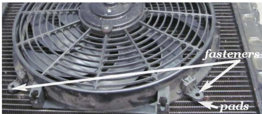
The plastic fasteners and the rubber pads are really not good enough. As plastic is more abrasive than copper the slight movement eventually allows contact with both and the copper loses.
