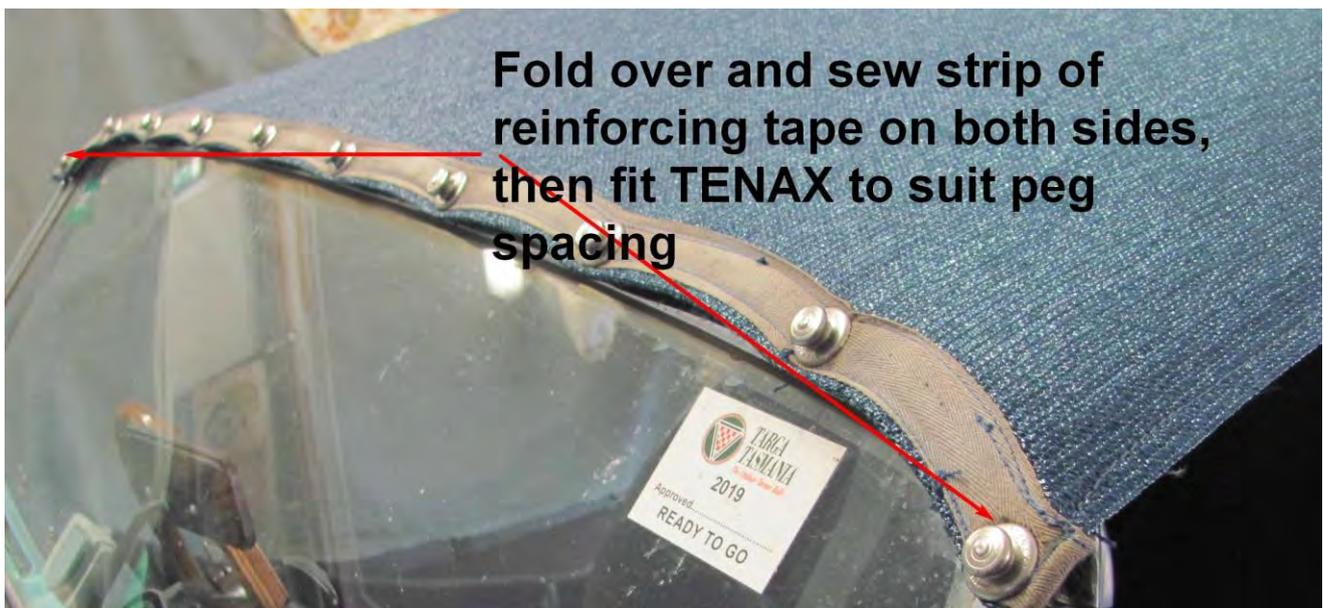
Having fixed the front to the windscreen frame it is time to stretch the cloth to the back and mark out the line for the same process as the front, fold over, sew tape on both sides ready for lift the Dots.
