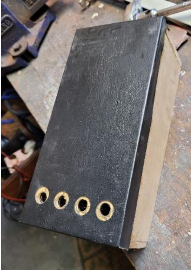
To make the box, I cut out cardboard templates for the front and back in cardboard. The main reason was to get the curve on the tunnel right. When I was happy with the template, I cut out the ends with a jigsaw. Used plywood. The rest was just making the sides and top to fit. I had some vinyl that I had used to make all the flat panels and dash so covered the top in the vinyl.
