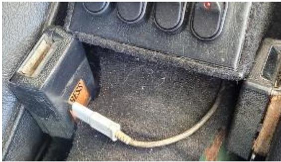
I ran a charger to the phone area. I wired up a cigarette lighter socket under the dash and bought a plug-in USB plug. I run a USB charging cable to the phone under the carpet.
