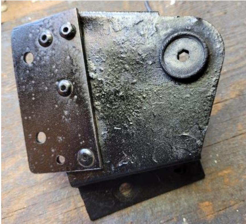
A problem you may encounter is that the mounting bracket has three attachment points to the body. One is a stud that goes through the firewall and has a nut behind the glovebox. Usually not a problem. The other two fit into captive nuts which are between the underside of the inner guard and the guard itself. When I took the bolts out, they had probably never seen the light of day for sixty years. One stripped. I had to put a nut under the captive nut in a space about 20mm wide.
