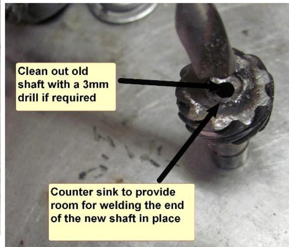
Now the shaft or old cable can be inspected and or removed. If the weld has failed and the square drive is still good, then just re weld.
