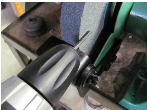
Fit the square end into your electric drill and use a running grind stone to turn it down to fit into the gearwheel.
