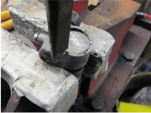
Fix the outer disc by burring over the edge with a chisel in 4 places, check that it turns freely and put it all back into the car.
