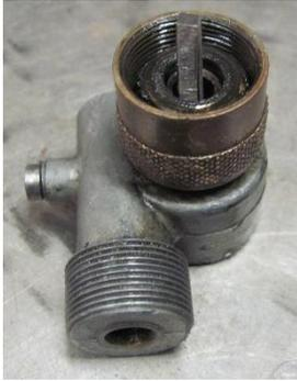
The first thing is to determine why it does not work. The most common issue is the rounding off of the male square drive shaft and sometimes it will be the connection between the drive shaft and the gear.
