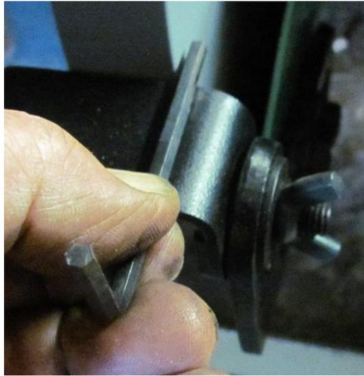
You will notice that the top and bottom flats provide a perfect reference surface on the grinder guide as you want to remove the 2 side of the Hex to produce a square.
