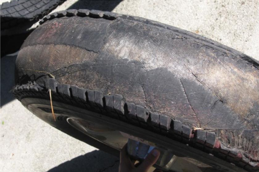
For years, people have relied on a tyre's tread depth to determine its condition. But the rubber compounds in a tyre oxidize and deteriorate with time, regardless of the condition of the tread. An old tyre poses a safety hazard.
