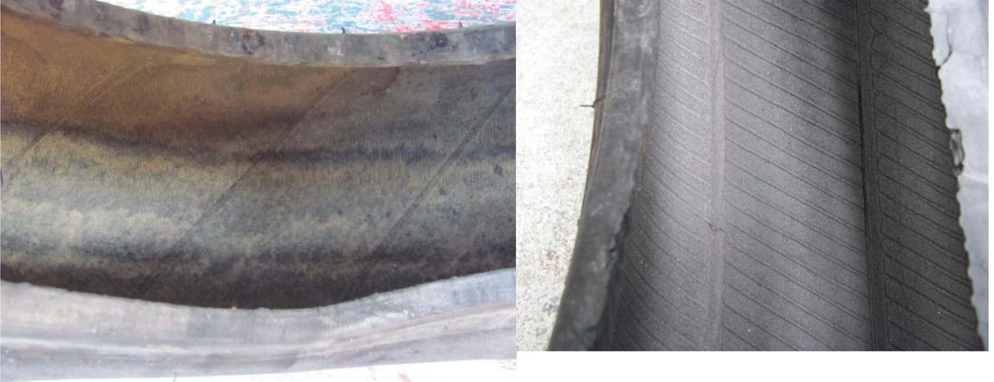
Tubes reduce the flexibility of tubeless tyres, and tubes tend to squirm around inside the casing as they flex under load thereby increasing rolling resistance and consuming a bit more energy and with the added internal friction this extra energy is turned into heat in the tyre. The heat will be sufficient to vulcanise the tube to the casing with almost certain failure.
